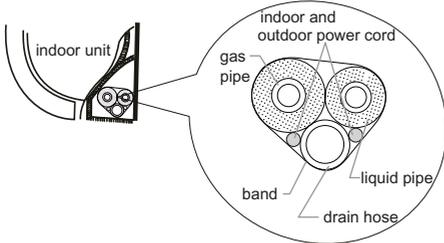
2. Reserve a certain length of drain hose and power cord for installation when binding them. When binding to a certain degree, separate the indoor power and then separate the drain hose.
