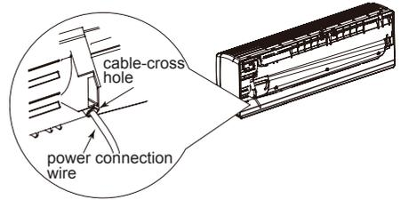
3. Remove the wire clip; connect the power connection wire to the wiring terminal according to the color; tighten the screw and then fix the power connection wire with wire clip. After finishing wiring of 18K unit, clamp the grounding wire (yellow-green wire) into the wire-crossing groove as shown in the following figure, in order to avoid pressing the wire when closing the electric box cover.
