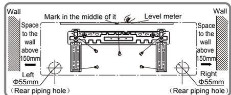
2. Open a piping hole with the diameter of  $\Phi 55$  on the selected outlet pipe position. In order to drain smoothly, slant the piping hole on the wall slightly downward to the outdoor side with the gradient of 5-10°.
