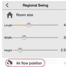
User can move the person icon among nine pane areas according to requirement to adjust the fan-blow area. The Regional Swing function can be turned off through up&down swing. The up&down swing in the Regional Swing is only valid under cooling and heating modes. The left&right swing area has relationship with the position of air conditioner set by mobile phone. The left&right swing position may be asymmetry, which is the normal phenomenon.
