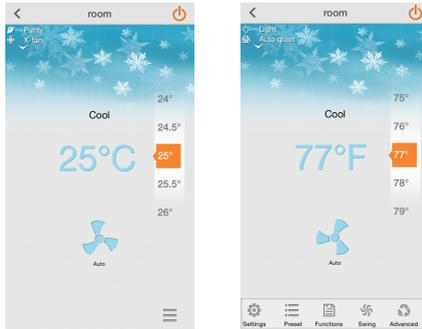
3. Fan Speed: It used for setting fan speed. Under cooling or heating mode, if the noise-customized function is turned on, adjust the fan speed and then the noise-customized function will be turned off automatically. Please refer to the part of remote controller for detailed operation.
